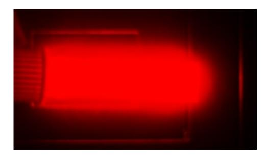
Bright light emission from silicon quantum dots in a cuvette. The image is from a camera that captures the near-infrared light that the quantum dots emit. The light emission shown is a psuedo color, as near-infrared light does not fall in the visible spectrum. Credit: Folarin Erogbogbo
