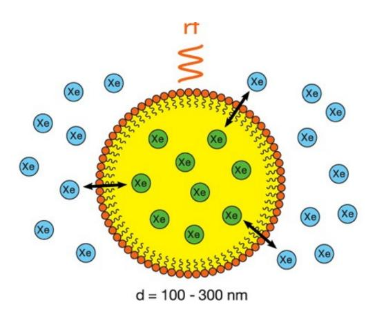
In this new NMR/MRI technique, hyperpolarized xenon gas bubbled into solution serves as the reporting medium as it moves in and out of a perfluorocarbon nanoemulsion droplet that binds to a molecular target. The contrast stems from the interaction of the distinguishable signals outside and inside the droplets.
