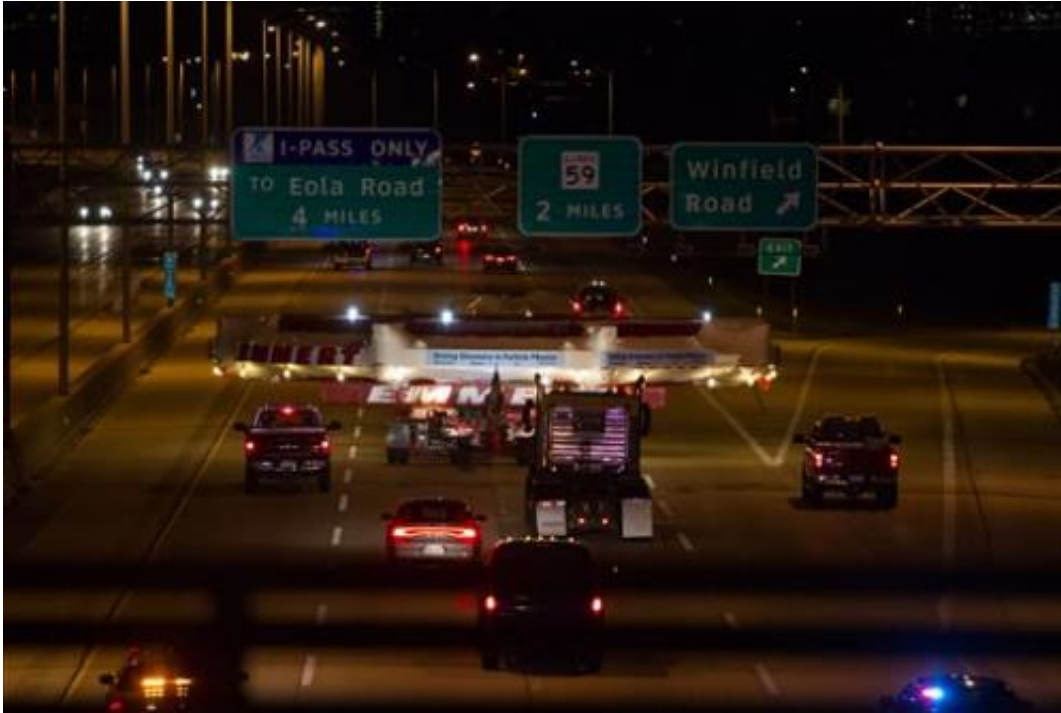
The electromagnet moves down Interstate 88 in Naperville, Ill., Friday, July 26, 2013 on its way to Fermilab. The electromagnet is 50 feet wide, weighs more than 15 tons and has taken a month to transport 3,200 miles from New York to Illinois. (AP Photo/Scott Eisen)
