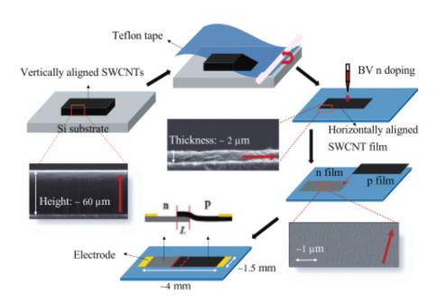
These schematic diagrams depict the fabrication process for p-n junction photodectors using flattened, highly aligned nanotube carpets. Credit: X. He/Rice University
