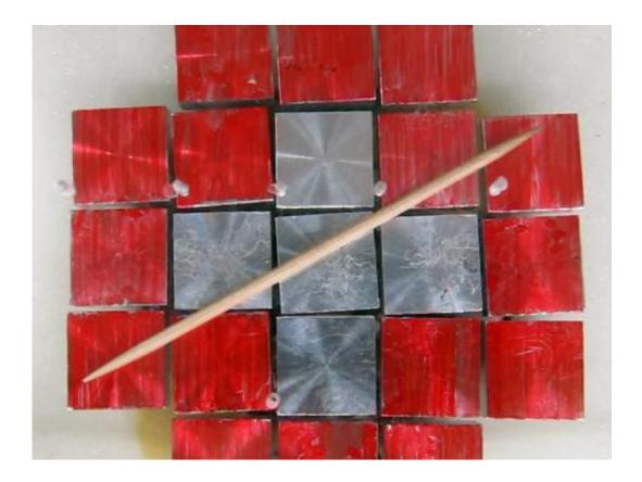
The researchers control the movement of levitated objects - here a toothpick - by varying the acoustic waves of several parallel emitter-reflector modules. Credit: Daniele Foresti / ETH Zurich
