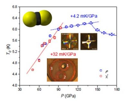
Pressure dependence of the critical superconducting temperature of a metal created by the team from CS2 molecule (top left) was measured be electrical contacts ( inset in the middle) and electromagnetic coils (inset at the bottom).
