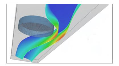
Placing a micropillar in a micro-channel causes flow to fundamentally change. By varying the size and location of the pillar, a rich variety of flows can be created. The figure shows a simulation of streamlines for one particular configuration run on TACC's Stampede supercomputer. Credit: Baskar Ganapathysubramanian, Iowa State University
