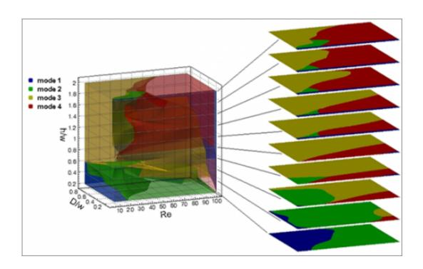
Exploring the phase space of fluid deformations using high throughput computing: Each configuration of microfluidic system (pillar diameter, channel height, and flow speed) results is a specific fluid deformation. XSEDE resources were used to classify these deformations. Such classification is fundamental to subsequent fluid sculpting.
