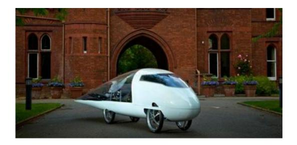
The 2013 solar car developed by Cambridge students has a more aerodynamic design, thanks to tracking solar panels at the back, which prevent any compromise on its shape. Credit: CUER
