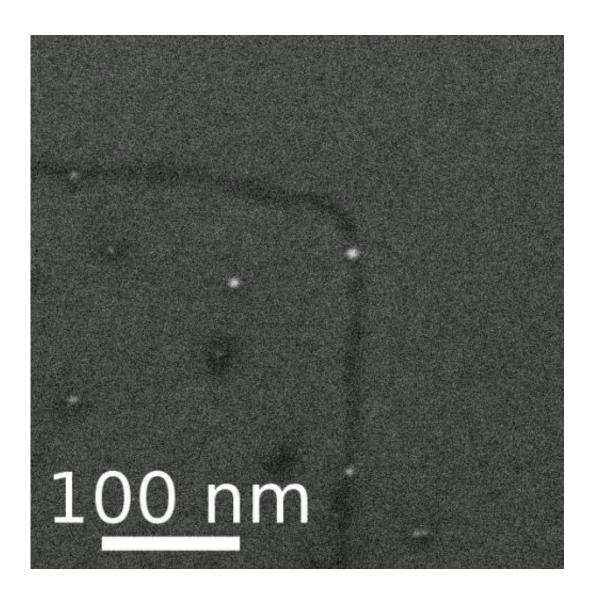
A graphene nanowire turns a corner. The nanowire was created via a process invented at Rice University in which a water layer only a few molecules thick acts as a mask. Credit: Tour Group/Rice University
