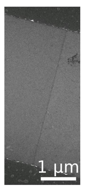
A thin line of graphene connects two electrodes in a test field-effect transistor built at Rice University. The graphene nanoribbons was created with a new process that depends on a meniscus mask a few molecules of water thick. Credit: Tour Group/Rice University
