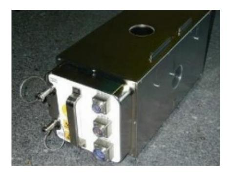
The high temperature insert is placed in the device for the study of critical liquids and crystallization. Credit: CNES
