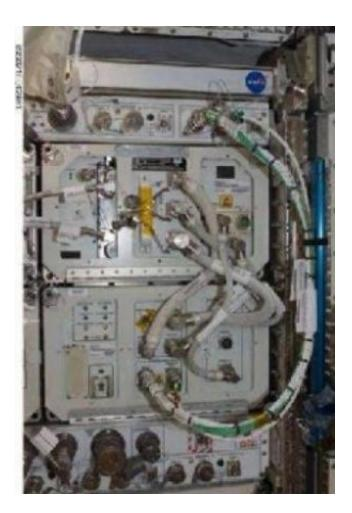
The Device for the Study of Critical Liquids and Crystallization has two rectangular boxes. The upper box contains the High Temperature Insert and all the diagnostic hardware. The lower box contains the command/control and data storage hardware. Credit: CNES
