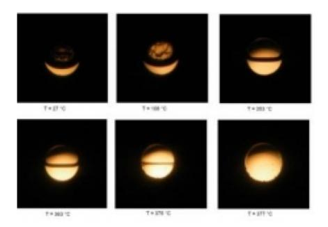
This shows images of water/saline solution being heated. The temperature and pressure increases through the critical point until there is no distinction between water's liquid and vapor phase. This is evidenced by the disappearance of the thin black line that separates the phases. Credit: NASA
