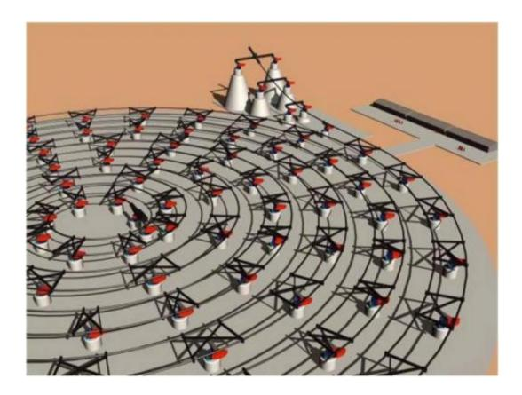
An artist's concept for a full scale Slingatron space launcher about 200-300 meters in diameter. The spiral track is mounted on support pylons which contain drive motors and counterweight flywheels. Payload assemblies are prepared for launch nearby.
