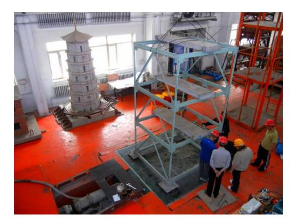
Earthquake-engineering researchers at the Harbin Institute of Technology in China work to set up a structure on a shake table for experiments to study the effects of earthquakes. Purdue University civil engineering students are working with counterparts at the institute to study the reliability of models for testing a type of powerful damping system that might be installed in buildings and bridges to reduce structural damage and injuries during earthquakes. Credit: Harbin Institute of Technology
