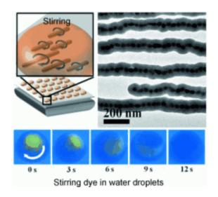
Anyone who has ever worked in a laboratory has seen them: magnetic stirrers that rotate magnetic stir bars in liquids to mix them. The stir bars come in many different forms—now including nanometer-sized. In the journal *Angewandte Chemie*, researchers from Singapore have now introduced chains made of 40 nm iron oxide particles that act as the world's smallest magnetic stir bars, effectively stirring picoliter-sized drops of emulsion with a commercial magnetic stirrer.
