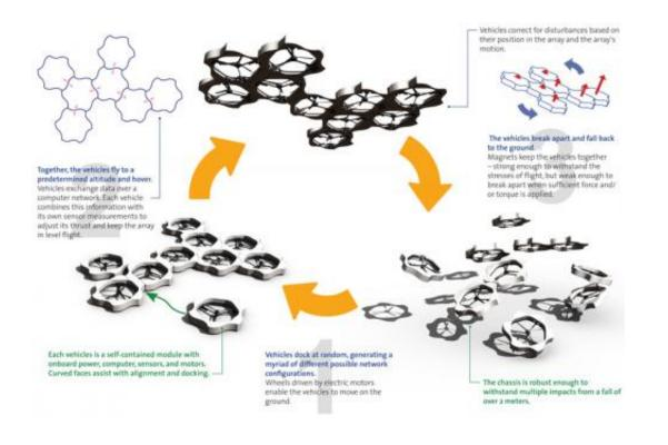
Researchers at ETH Zurich, a technical University in Switzerland, have developed a unique type of copter. It's made of several single rotor craft that physically connect to one another autonomously to create a larger multiple rotor craft. Because the craft is self-assembled, each time it takes flight, it has a different configuration. The researchers call their craft a Distributed Flight Array (DFA).
