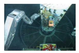
The image above shows ROV Jason's arm manipulating a pressure measurement system on the wellhead of the borehole observatory during the summer 2011 expedition. Images below show fluid sampling activities carried out by ROV Jason during the summer 2011 expedition.
