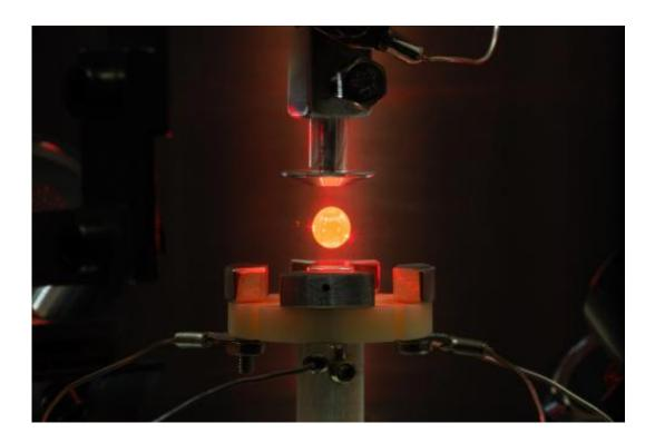
The hot droplet is suspended in a vacuum between two electrodes. While the droplet cools down or is heated up, its structure is continuously monitored by exposing it to radiation from the synchrotron source. Credit: Institute of Materials Physics in Space at the German Aerospace Centre (DLR) in Cologne, Germany.
