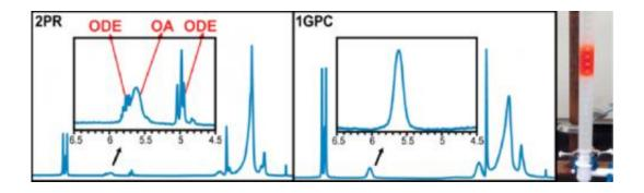
Purification of semiconductor quantum dots is much more effective with gelpermeation chromatography that with the traditional precipitation-redissolution technique. Credit: American Chemical Society
