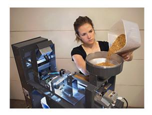
Biological science aide Anne Berry puts wheat in the hopper of a color-image sorter. The ARS-developed camera behind her takes and processes a color image of each kernel as it falls off the end of the chute. The kernels are then sorted based on visual features and deposited into either of two separate buckets at the base of the sorter. Credit: Thomas Pearson.
