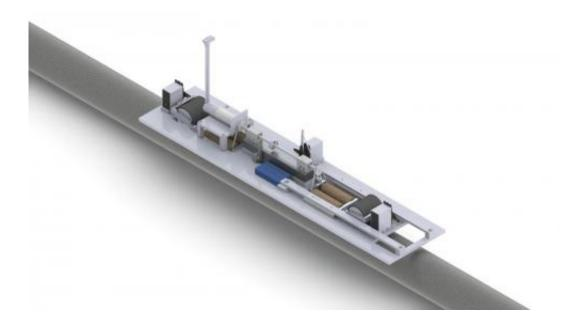
CAD model of the robot inspecting a wire cable. Credit: Fraunhofer IZFP
