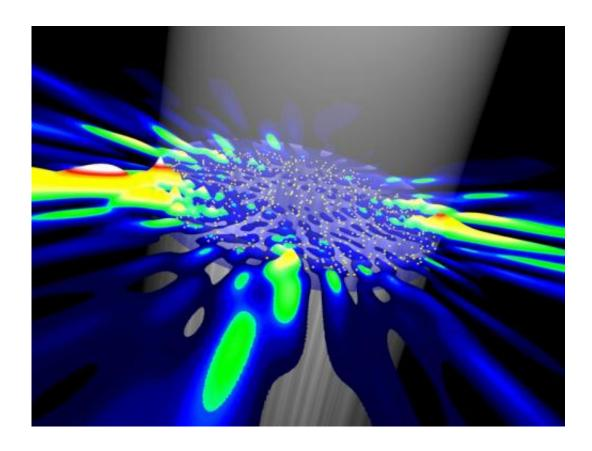
Random lasers are powered by a beam of light from above. Random scatterers inside the laser (yellow dots) lead to chaotic emission of light into all directions.
