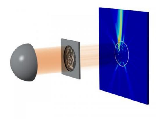
Here, the beam of light is first sent through a mask, so that different regions of the laser are pumped with different amounts of energy. This selectiv pumping leads to the laser emitting a beam of light exactly into the right direction.
