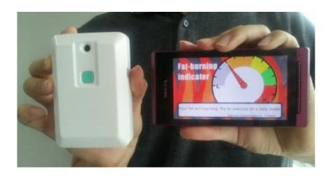
This shows a portable breath acetone analyzer and an Android-based smartphone for displaying results. Credit: NTT DOCOMO
