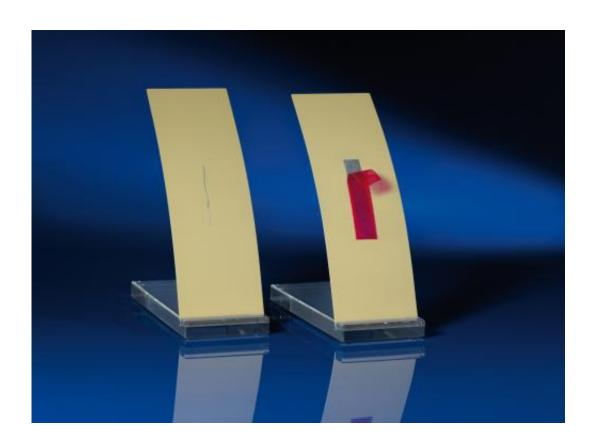
Application of pickling tape prior to the repair of damaged paint. The paint has been removed by mechanical abrasion and the pickling tape is used for pretreatment of the metal surface. After removal of the tape and simple cleaning with a damp cloth, the surface is ready to receive a fresh coat of paint. Credit: Fraunhofer IFAM
