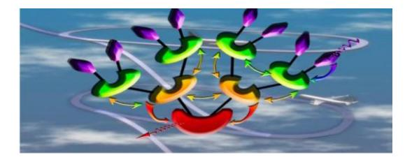
Illustration of the light-harvesting funnel array that directs energy to a focal point along diverse routes, and then slowly off-loads the energy to a solar cell or other device. Credit: Raymond Ziessel, et al. ©2013 American Chemical Society
