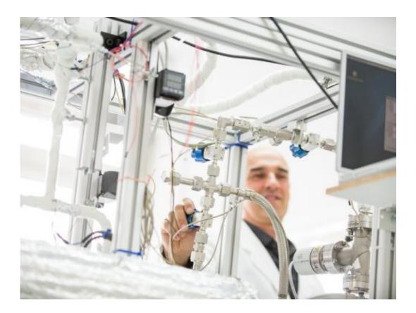
An important part of the Arktis technology: the gas handling system, preparing the gas in a several-step process before filling. Credit: Arktis Radiation Detectors
