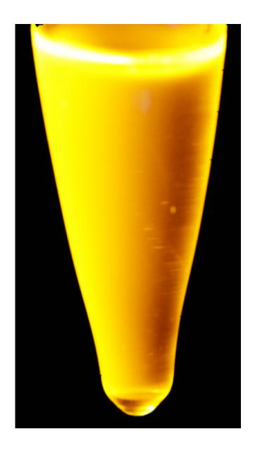
A solution containing millions of manganese-doped quantum dots in a plastic container glows orange. Credit: APS
