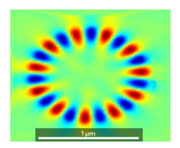
An efficient FDTD simulation can quickly calculate the electric and magnetic field patterns inside a nanocavity laser. Credit: IEEE
