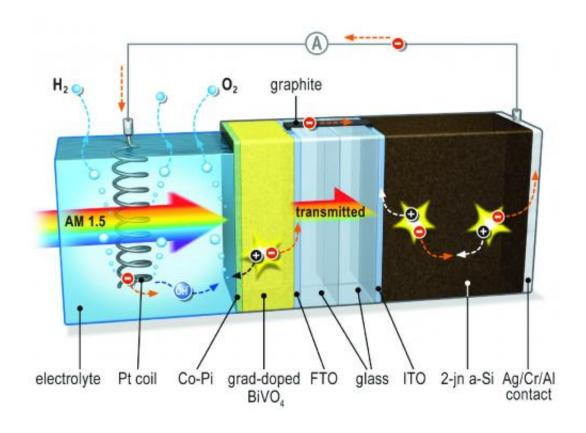
When light hits the system, an electrical potential builds up. The metal oxide layer acts as a photo anode and is the site of oxygen formation. It is connected to the solar cell by way of a conducting bridge made of graphite (black). Since only the metal oxide layer is in contact with the electrolyte, the silicon solar cell remains safe from corrosion. A platinum spiral serves as the cathode where hydrogen is formed. Credit: Image: TU Delft
