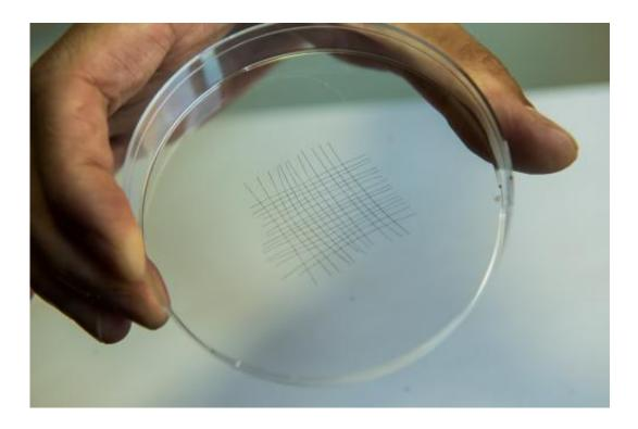
Rice University graduate student Changsheng Xiang spun fibers from graphene oxide flakes. The fibers are as strong at knots as anywhere along their length and should be suitable for weaving into advanced fabrics. Credit: Jeff Fitlow/Rice University
