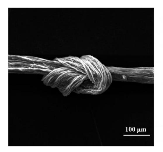
A knotted carbon fiber made at Rice University has the same tensile strength along its entire length. That property may make it suitable for advanced fabrics. Credit: Tour Group/Rice University
