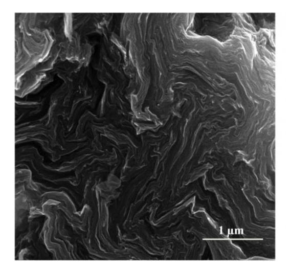
Flakes of graphene oxide are the major component in a new process invented at Rice University for making carbon fiber. The two-dimensional flakes align in a wet spinning process and are held together by the Van der Waals force. Credit: Tour Group/Rice University
