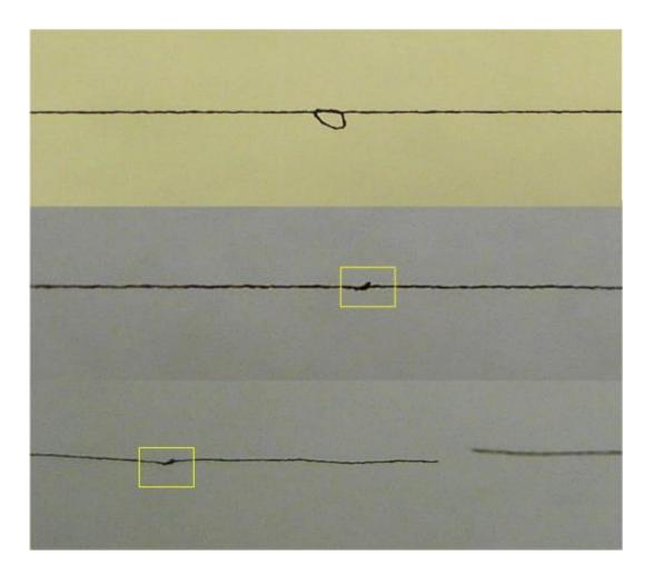
A knotted carbon fiber created at Rice University breaks along its length and not at the site of the knot, unlike most other fibers. The knots achieve "100 percent efficiency" due to the use of graphene oxide flakes. Credit: Tour Group/Rice University
