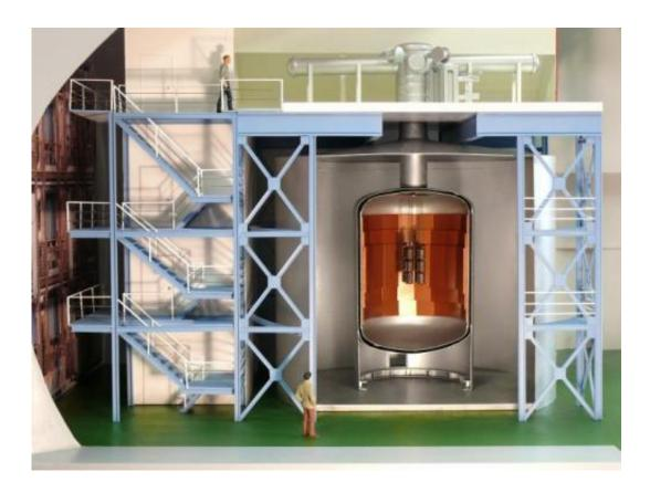
This model of the GERDA experiment shows the onion-like structure which suppresses interfering signals from the environment. The germanium diodes in the center of the cryostat filled with liquid argon  $(-186^{\circ}C)$  are to a larger scale. Credit: MPI for Nuclear Physics
