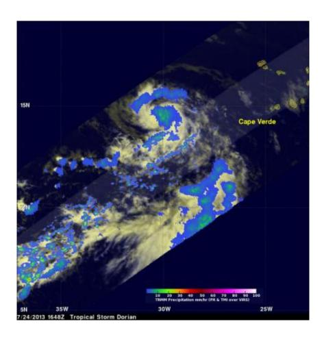
NASA's TRMM satellite flew over tropical storm Dorian on July 24 at 1648 UTC and the TMI and PR instruments saw light to moderate rainfall (blue/green)
