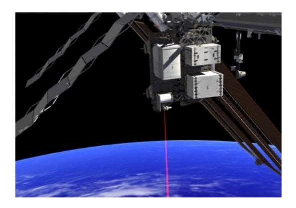
This artist's concept shows how the Optical Payload for Lasercomm Science (OPALS) laser will beam data to Earth from the International Space Station. Credit: NASA.
