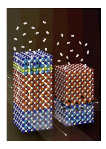
Researchers from MESA+, the research institute for nanotechnology at the University of Twente, have developed a method to reduce the number of 'defects' in heterogeneous oxide materials. As a result, the
