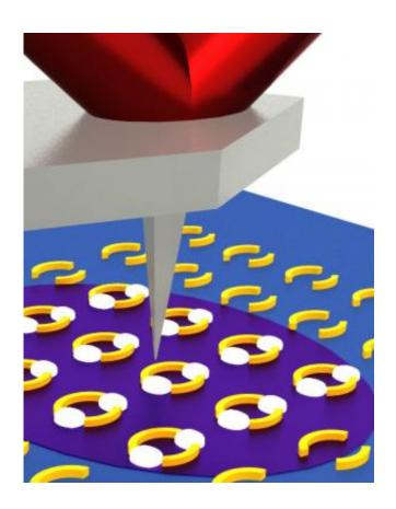
Infrared laser light (purple) from below a sample (blue) excites ring-shaped nanoscale plasmonic resonator structures (gold). Hot spots (white) form in the rings' gaps. In these hot spots, infrared absorption is enhanced, allowing for more sensitive chemical recognition. A scanning AFM tip detects the expansion of the underlying material in response to absorption of infrared light. Credit: NIST
