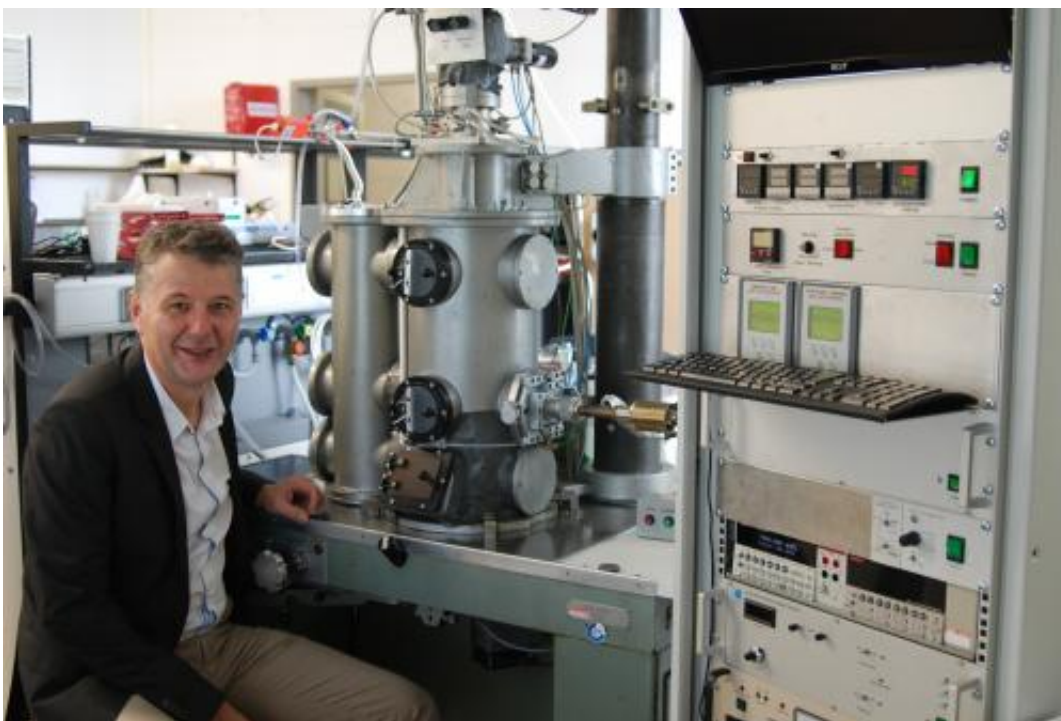
Professor Dr Norbert Mitzel with the improved gas electron diffractometer.
