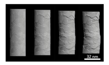
Simulated deformation of a platinum nanopillar under increasing levels of compression from left to right. Credit: 2012 American Chemical Society
