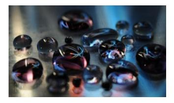
Research conducted at the Institute of Physical Chemistry of the Polish Academy of Sciences and the Institute of Physics of the PAS revealed that tiny temperature differences – even as small as ten-thousandths parts of kelvin – are the primary driving force in droplet evaporation.Credit: IPC PAN, Grzegorz Krzyżewski
