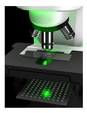
Artist's rendering of the microscopy setup showing one element of an LED array illuminating a sample. Credit: Yan Liang and Guoan Zheng
