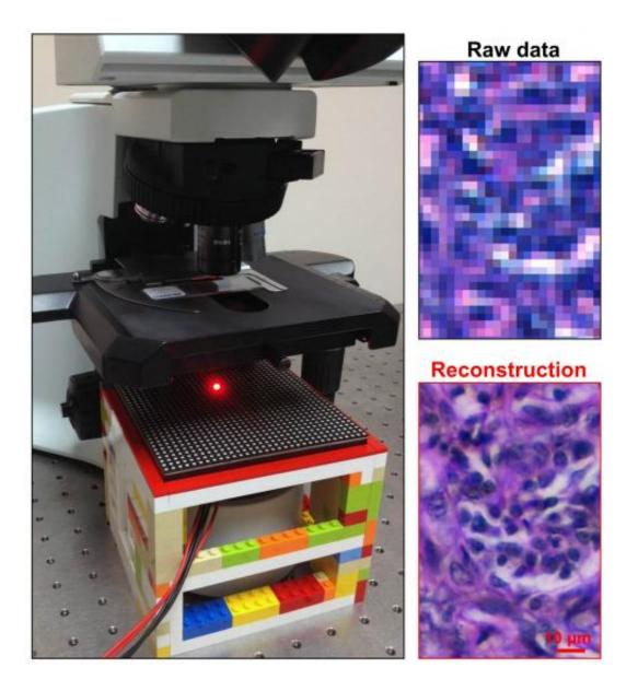
Changhuei Yang's lab at Caltech has developed a new microscope setup (left) that converts a relatively inexpensive conventional microscope into a billionpixel imaging system that significantly outperforms the best available standard microscope. A raw image taken with a 2X objective lens is shown (top right) along with the reconstructed image produced by the new microscope setup (bottom right). Credit: Guoan Zheng
