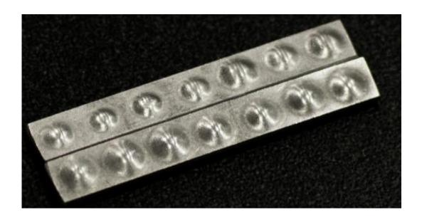
Researchers at North Carolina State University have developed a new metallic bubble wrap that is lighter, stronger and more flexible than sheet metal and more heat- and chemical-resistant than plastic or other polymer-based bubble wraps. Credit: Afsaneh Rabiei
