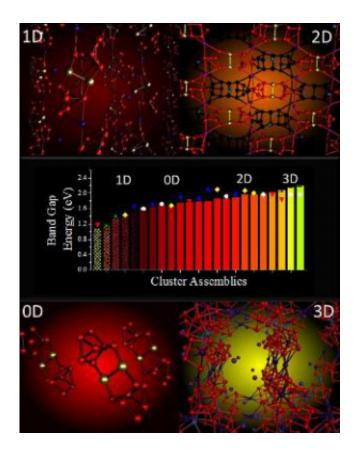
Cluster assembled materials with zero to three dimensional architectures, and the background color corresponds to the band gap energy of the material. The center graph shows the band gap energy of 23 cluster assembled materials synthesized in the study with the color corresponding to the band gap energy of the material. Credit: Arthur Reber Ph.D./VCU
