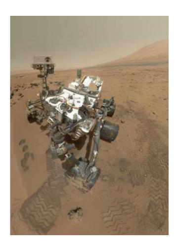
NASA's Curiosity rover used the Mars Hand Lens Imager (MAHLI) to capture this set of 55 high-resolution images, which were stitched together to create this full-color self-portrait. Credit: NASA/JPL-Caltech/Malin Space Science Systems
