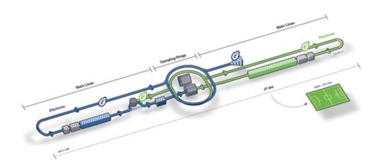
A schematic of the proposed International Linear Collider, which includes the damping rings designed by Cornell physicists. Credit: linearcollider.org
