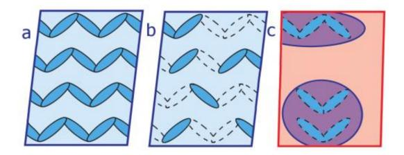
In its insulating state, the magnetite sample has electrical charges locked into structures known as "trimerons" that are composed of three iron atoms (a). An optical laser pulse was used to fracture trimerons (b), creating strands of electrical conductivity (red) surrounding islands of non-conducting trimeron structures (c). Credit: S. de Jong et al./Nature Materials
