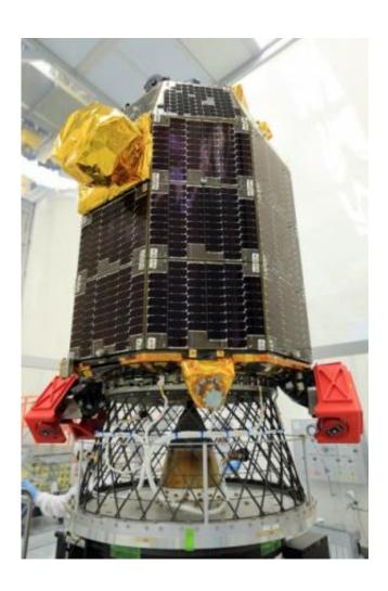
The LADEE spacecraft awaits spin balance testing, conducted to ensure stability during flight, at NASA's Wallops Flight Facility in Virginia. LADEE is slated to liftoff from Wallops on Sept. 5, 2013. Credit: NASA/Patrick Black
