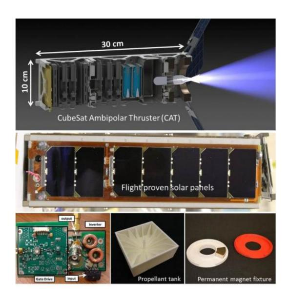
The CAT engine with the avionics, power system, propellant tank, magnetic nozzle, plasma discharge chamber, and solar panels.
