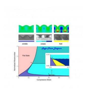
A phase diagram shows the amount of compressive strain needed to create wrinkles, creases and folds in rubbery materials. The purple area denotes the wrinkle state and the aqua areas are two crease states. The spot marked "R" denotes folding. The findings will help engineers control these states and use them in structured nanomaterials. Credit: Kim Lab / Brown University
