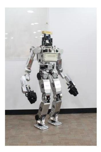
DRC-HUBO can switch from bipedal to quadrupedal walking, which provides the robot with greater stability to walk on uneven terrain or to climb up a hill. Credit: KAIST HUBO Lab & Rainbow Co.
