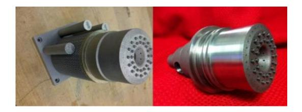
Left: 3-D printed rocket injector as it looked immediately after it was removed from the selected laser melting printer. Right: Injector after inspection and polishing. Credit: NASA/MSFC
