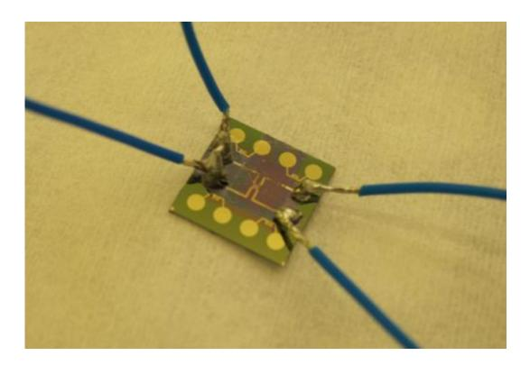
An electronic component where a graphene layer has been placed on the hotspots.
