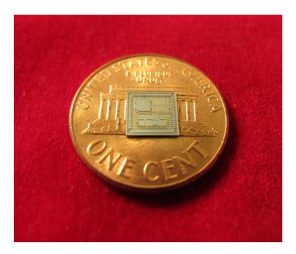
This tiny "timing inertial measurement unit" could take over when GPS is unavailable. Credit: Becky Peterson
