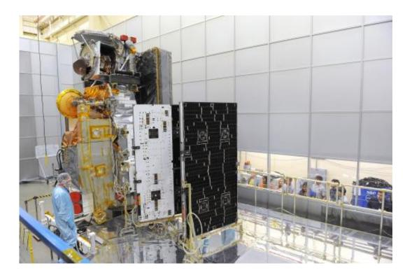
A solar array wing begins to release from the GPM Core satellite in a deployment test on Thursday, June 6, 2013. Credit: NASA Goddard/Debbie McCallum
